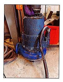
Over the last several weeks the maintenance staff noticed Pump 2 becoming noisy while running. This is often due to worn out bearings or an issue with the impeller. The pump was removed from service to be diagnosed and repaired. A spare pump was installed and placed into service.
