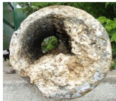
Result of Grease in Sewer Pipe
