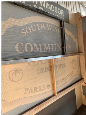
Mike Hanrahan sandblasting our new prototype signs out of sign foam. He is adding a wood grain texture by having a wire frame in front of the foam. We will be making more for our new Park Property as seen here - Deming gardens.
