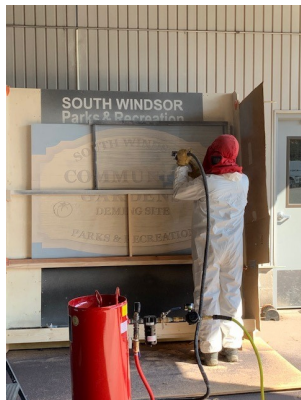
Mike Hanrahan sandblasting our new prototype signs out of sign foam. He is adding a wood grain texture by having a wire frame in front of the foam. We will be making more for our new Park Property as seen here - Deming gardens.
