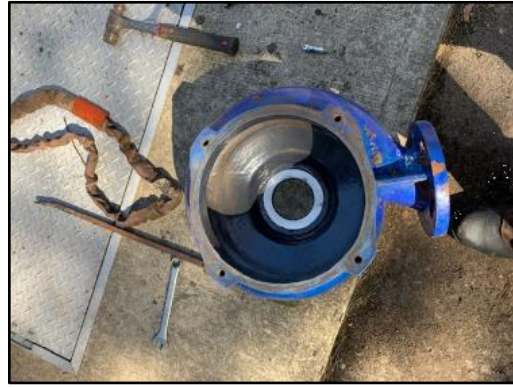
Top view of a volute which houses the pump impeller.
