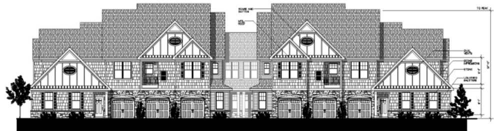
Building Type A - Front Elevation Scale 1/8"=1'-0"
