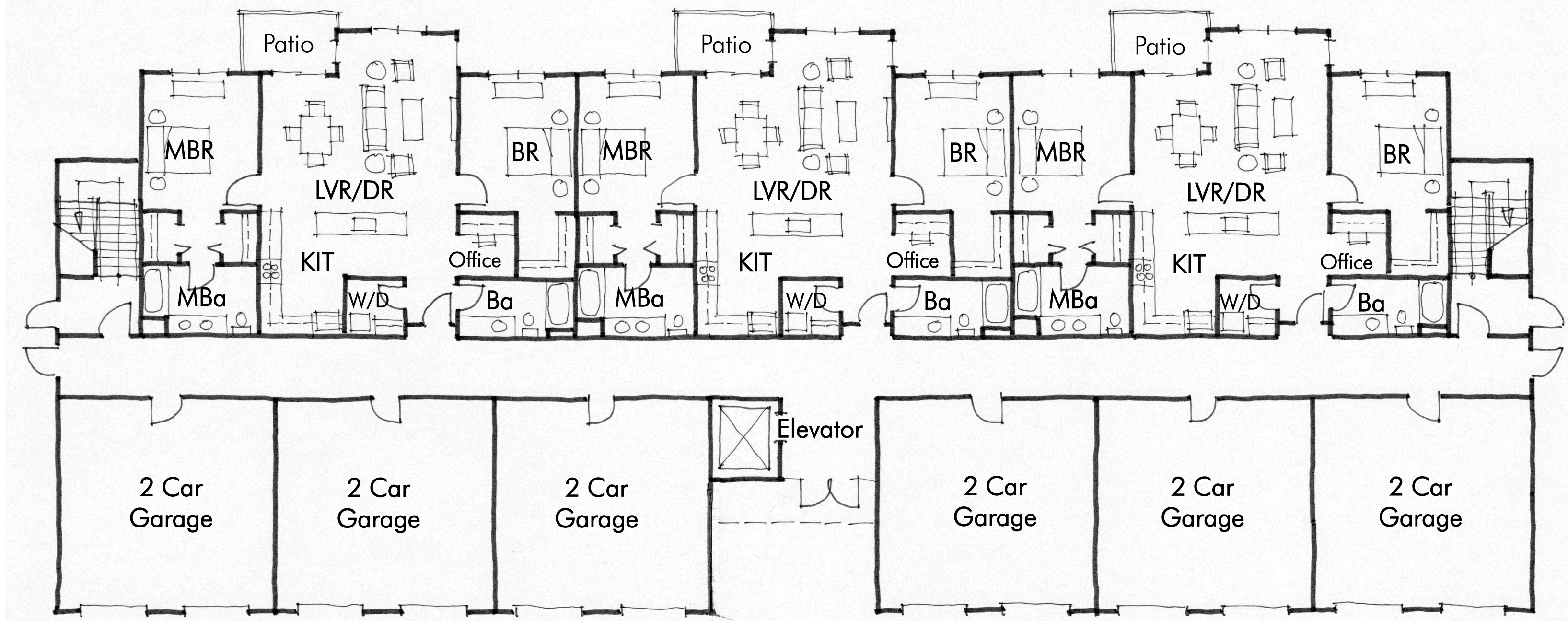
Unit #3 – First Floor Plan Floor Area = 8,550 SF Total Building Area = 14,050 SF Total (6) – 2 BR Units @1,350 SF each
