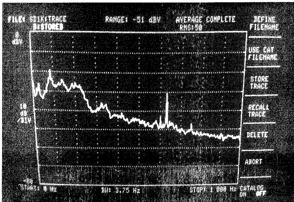
Figure 8. Discrete Tones Produced by the Fuel Cell Cooling Module (0 dBV = 88.6 dB re20μPa)
