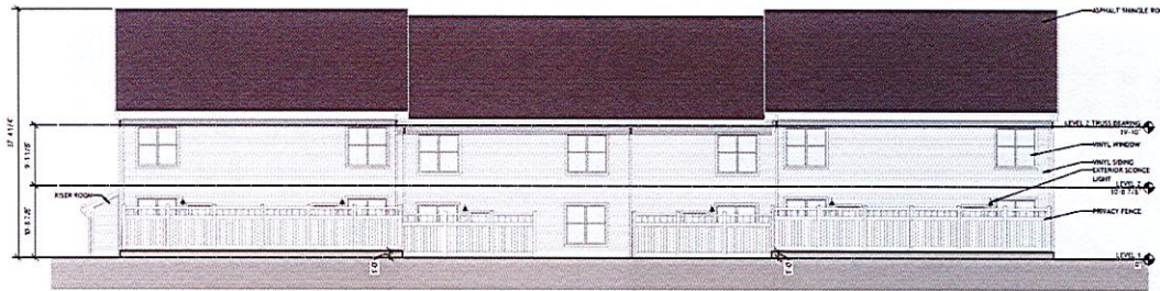
4 BUILDING ELEVATION - BUILDING TYPE C A3-03 1/8" = 1'-0"
