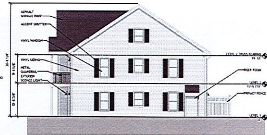
2 BUILDING ELEVATION - BUILDING TYPE B A3-02 1/8" = 1'-0"
