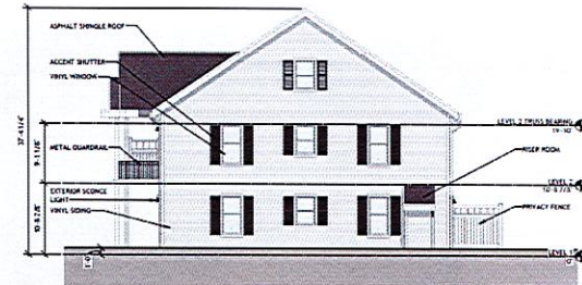
2 BUILDING ELEVATION - BUILDING TYPE C A3-03 1/8" = 1'-0"
