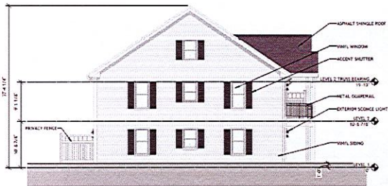
3 BUILDING ELEVATION - BUILDING TYPE C A3-03 1/8" = 1'-0"
