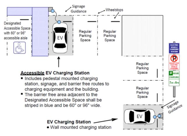
Figure 11.8A – EV Charging Station Design, including Accessible EV Charging Stations
