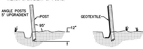
3. EXTEND GEOTEXTILE INTO TRENCH. 4. BACKFILL TRENCH AND COMPACT EXCAVATED SOIL.
