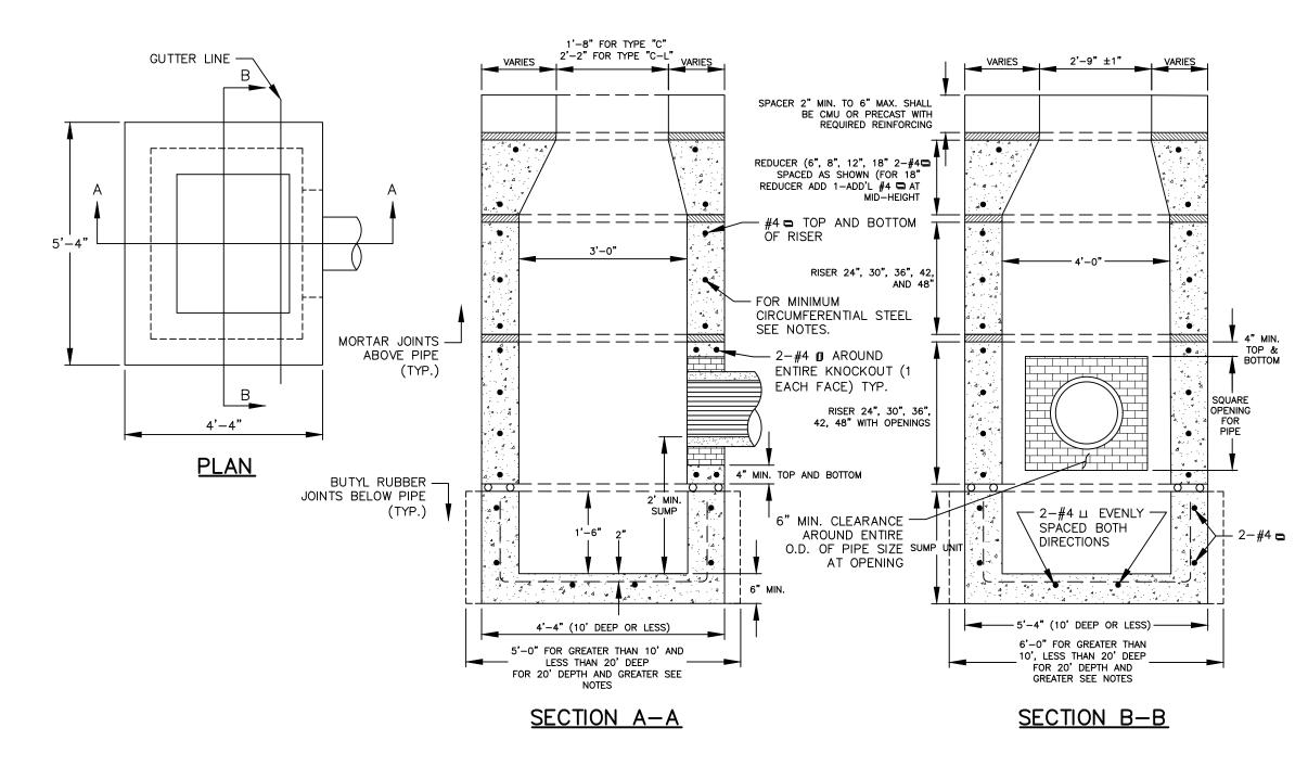
PRECAST CONCRETE TYPE "C" AND "C-L" CATCH BASIN
