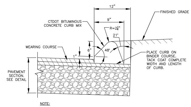
BITUMINOUS CONCRETE CURBING SHALL BE INSTALLED PER CTDOT STANDARD SPECIFICATIONS FOR ROADS, BRIDGES, FACILITIES AND INCIDENTAL CONSTRUCTION, LATEST EDITION.
