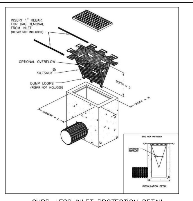
CURB-LESS INLET PROTECTION DETAIL
