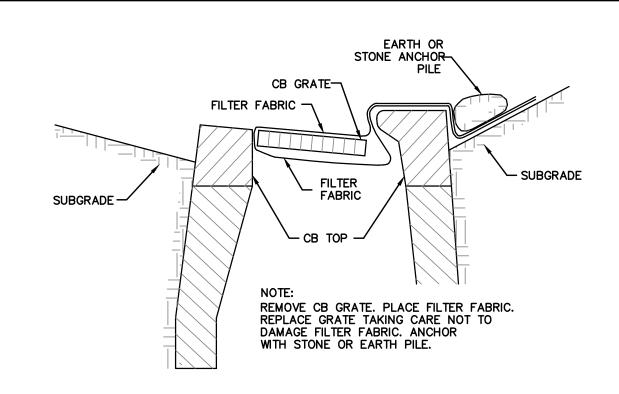
CATCH BASIN GRATE SEDIMENTATION CONTROL N.T.S.
