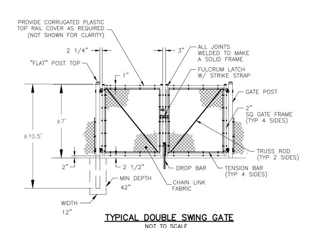
ALL FENCE COMPONENTS SHALL BE BLACK PVC COATED PROVIDE DROP BAR FOR EACH GATE & GROUND INSERT TO STABILIZE GATES IN BOTH CLOSED & OPEN CONDITIONS. PROVIDE LATCH POSTS TO STABILIZE GATES IN OPEN POSITION IF GROUND ELEVATIONS VARY.
