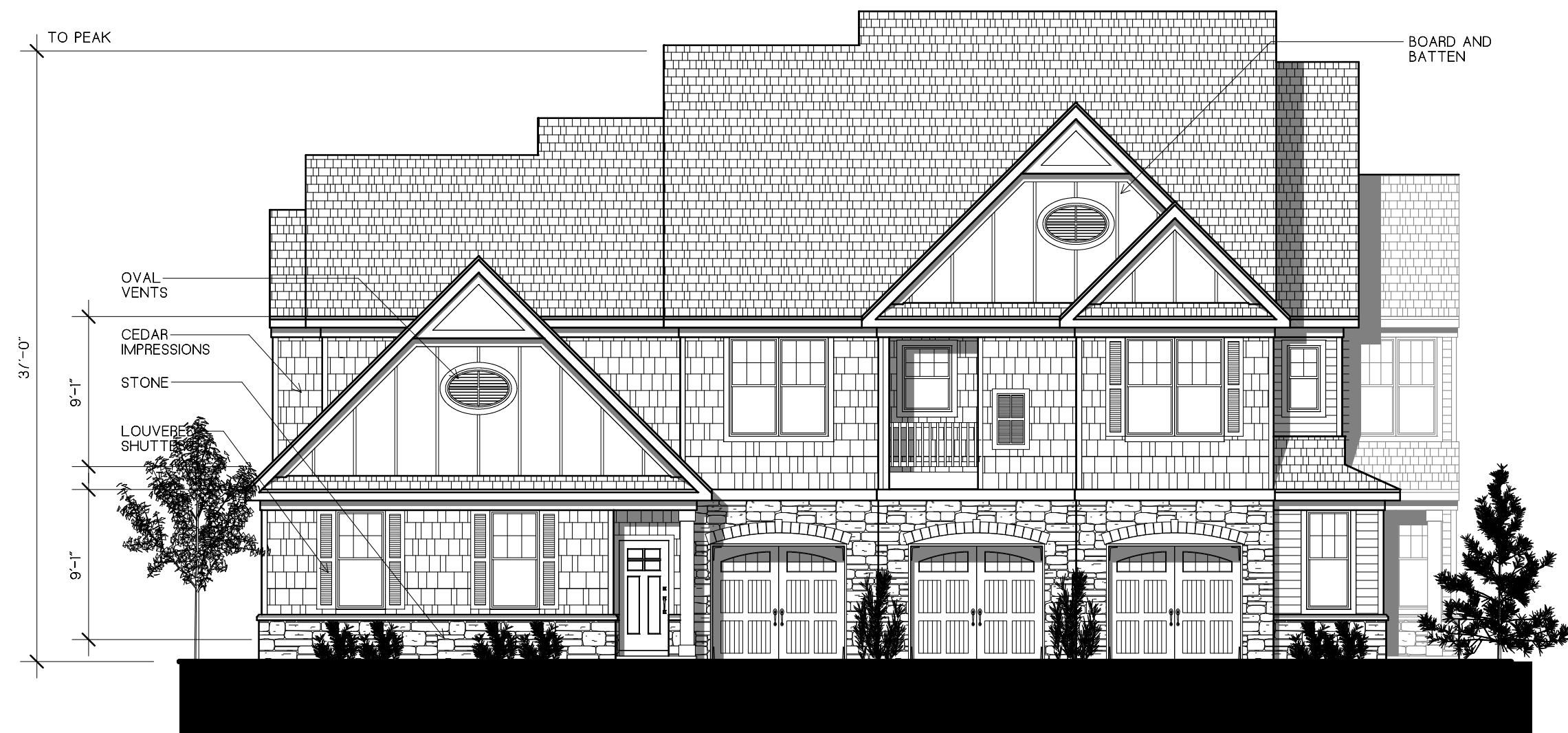
Building Type C - Front Elevation Scale: 1/8"=1'-0"
