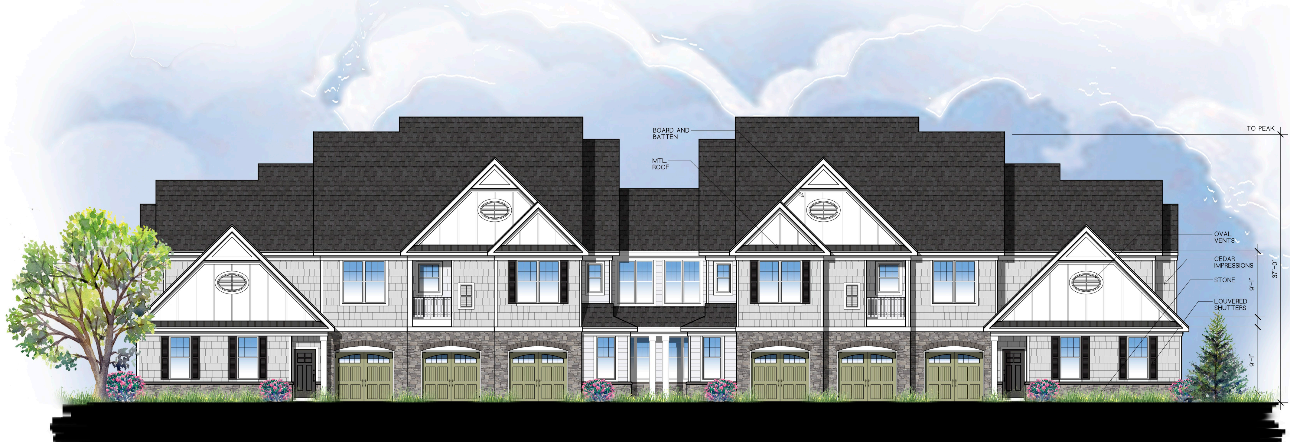
Building Type A - Front Elevation Scale: 1/8"=1'-0"
