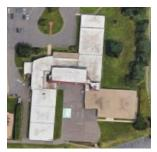
DescriptionTotal Estimated Project Cost: \$ 223,500.00Total Estimated Offset Funding: \$ NoneReplace roof with a Modified Bitumen roofing system covering approximately 10,214 sq.ft.
